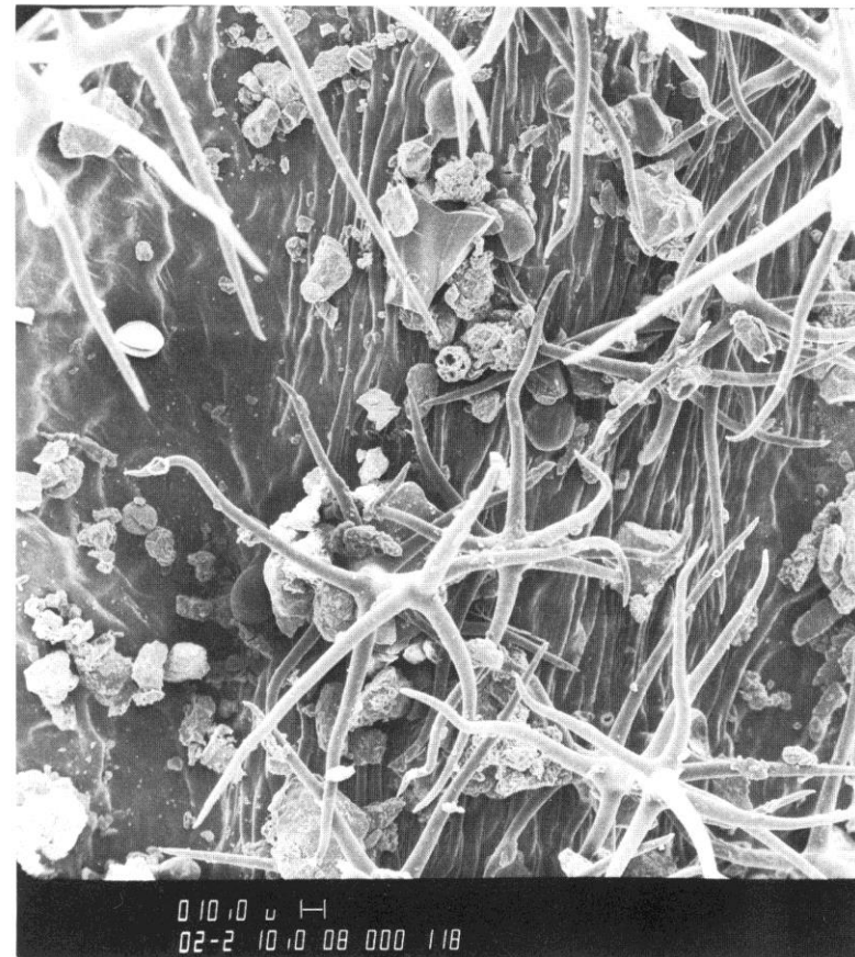
Figure 5-3. Scanning electron microscope micrograph of the adaxial surface of an 8-week-old London plane leaf. Spore, pollen, carbonaceous, angular, and aggregate particles are visible. Scale, 10 \mu m.
